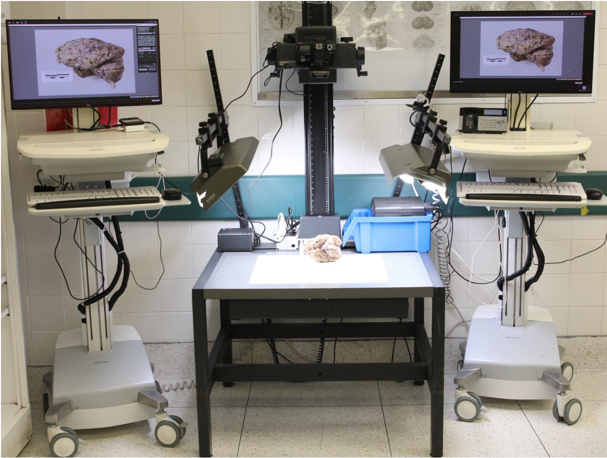
Figure 1. Forensic Teleneuropathology Setup for Remote Viewing of Brain Gross Examination
